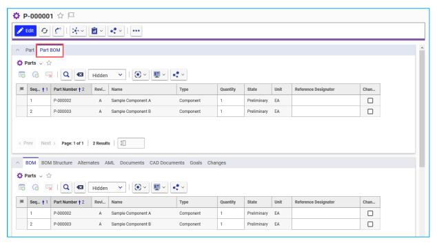
Figure 35. The Part BOM tab is added to the top accordion on the Part item view
