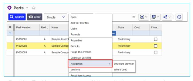
Figure 22. The default structure browser and where used actions appear in a new submenu
